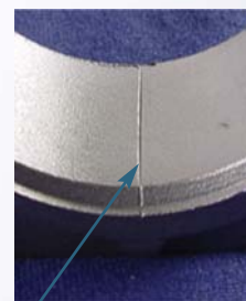
Minimize Machining Operations Forged Fracture Split Notch
