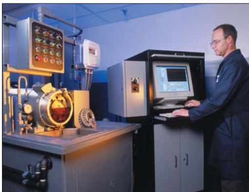
One-way clutch stroker test machine at the Romulus, Michigan Tech Center
